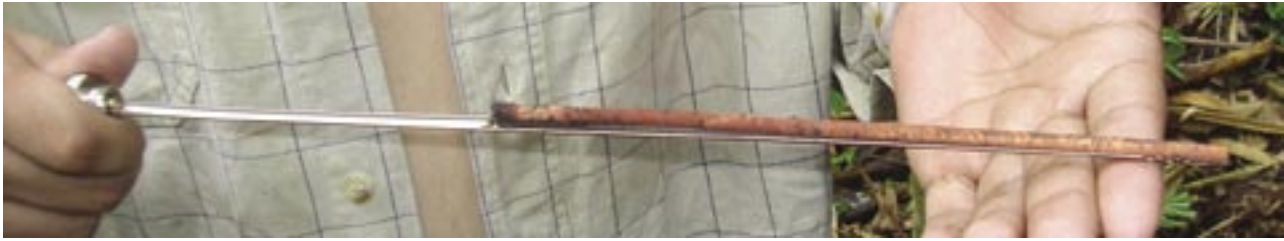
Heart rot: A timber sample of a standing mahogany tree obtained with the Pressler borer. Photo: I. Lombardi
