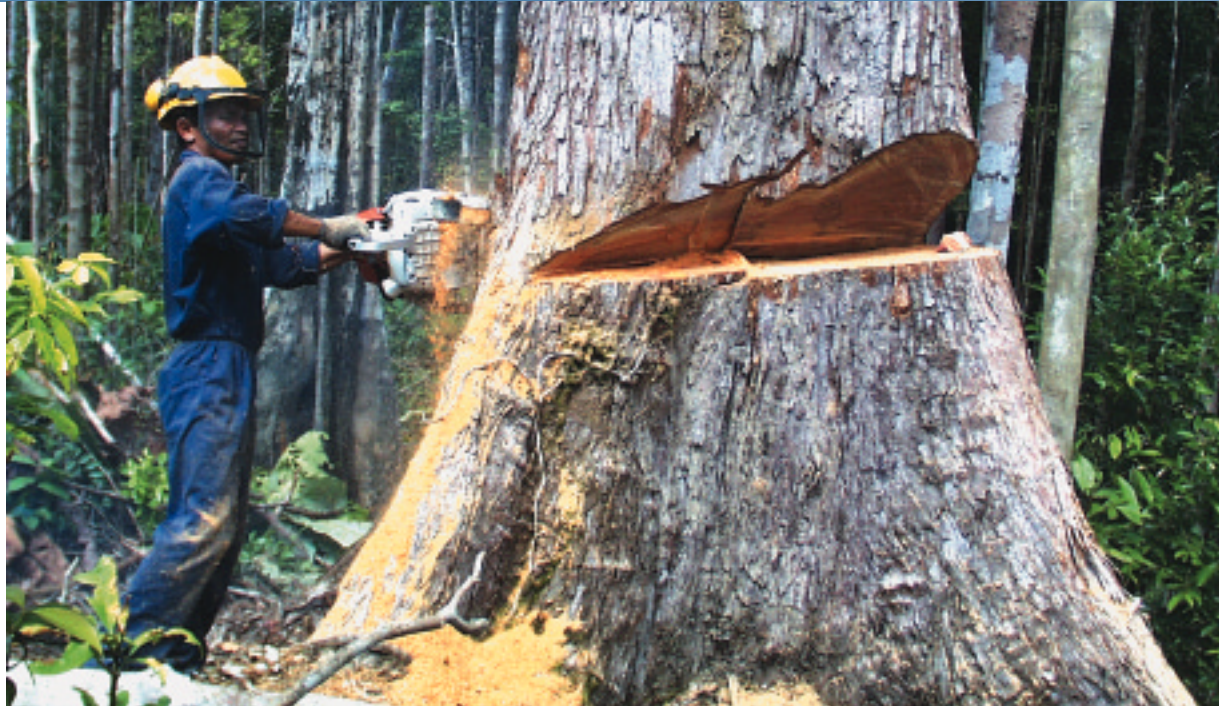
Which way? Directional felling is one of the components of RIL and requires on-the-job training. Photo: A. Hinrichs
