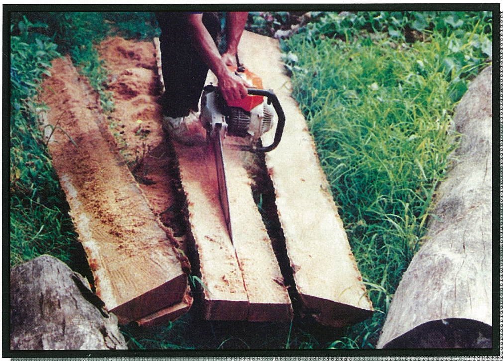
Chainsawing of coconut trunks into lumber
