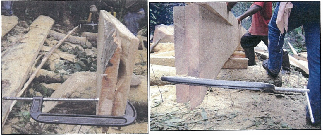
Figure 18: Edging of boards using C-clamps
