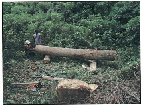
Figure 14: Logs resting on two wooden poles with wedges to facilitate milling
