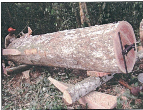
Figure 14: Logs resting on two wooden poles with wedges to facilitate milling
