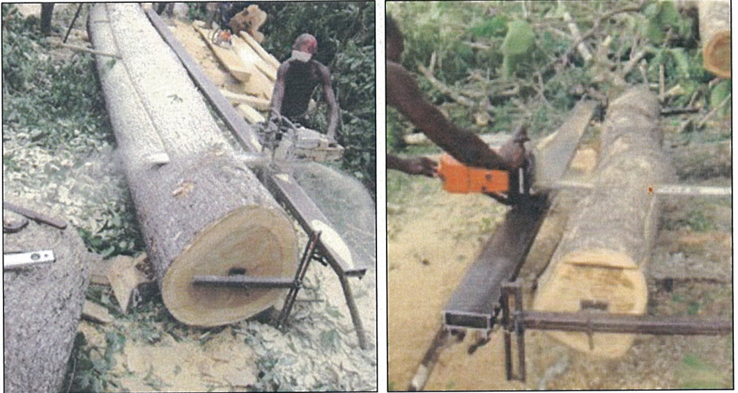
Figure 15: Milling of logs with Bigmill Basic to make the 1st cut
