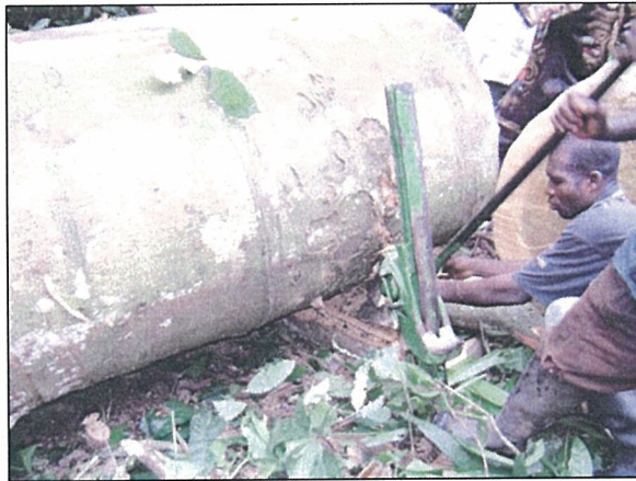
Figure 13: Using a timber jack to turn a log
