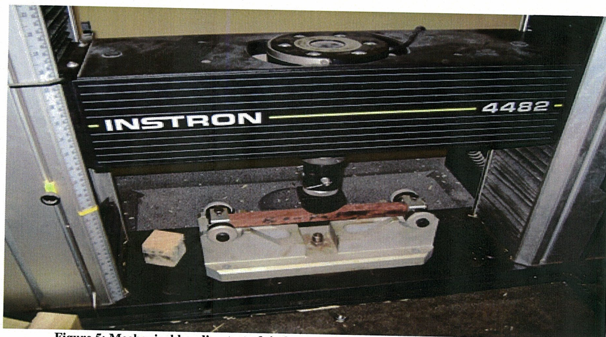
Figure 5: Mechanical bending test of timber species with universal Instron machine
