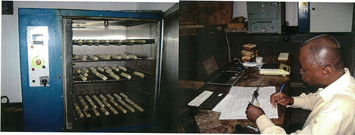
Figure 4: Scientist at work on the physical properties kiln schedules of some wood species
