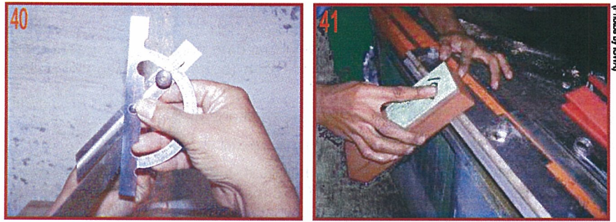
Figs 40-41 Measuring of knife blade angle (40); and double-bevel knife making (41)
