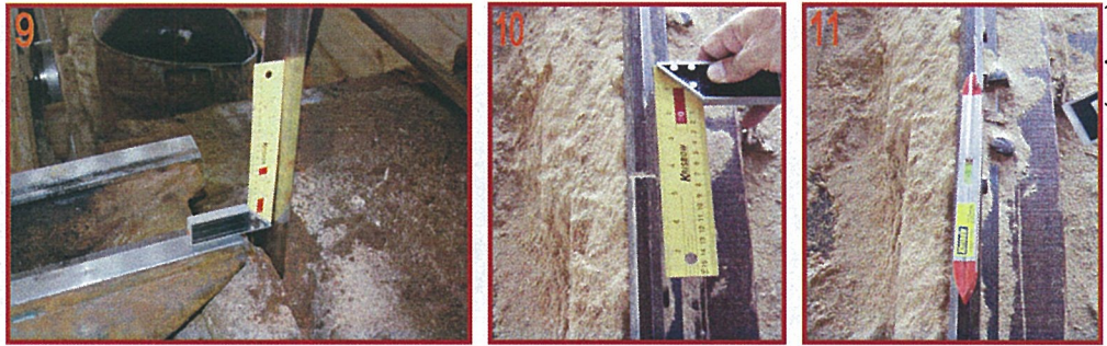
Figures 9-11. Fork head and band saw not perpendicular (9); rails not straight (10); rails not leveled (11)
