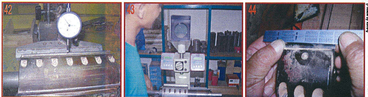
Figures 42-44. Measuring height of knives using micrometer (42), using optic machine (43) and measuring evenness of knives using special ruler (44).
