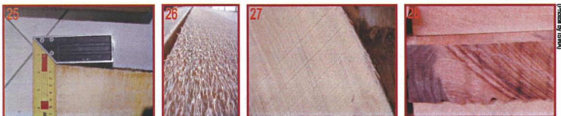
Figures 25-28. Angled sawn timber (25); fuzzy surface (26); sawmark (27); and saw burn (28)
