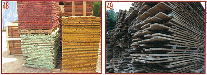
Figures 48-49. Sticks are the same as the wood to be dried (48); random stacking (49)
