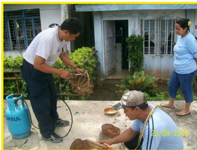
28. Study Leader Rodelio Mendoza's demonstration on the proper use of blow torch to clean up the finish product
