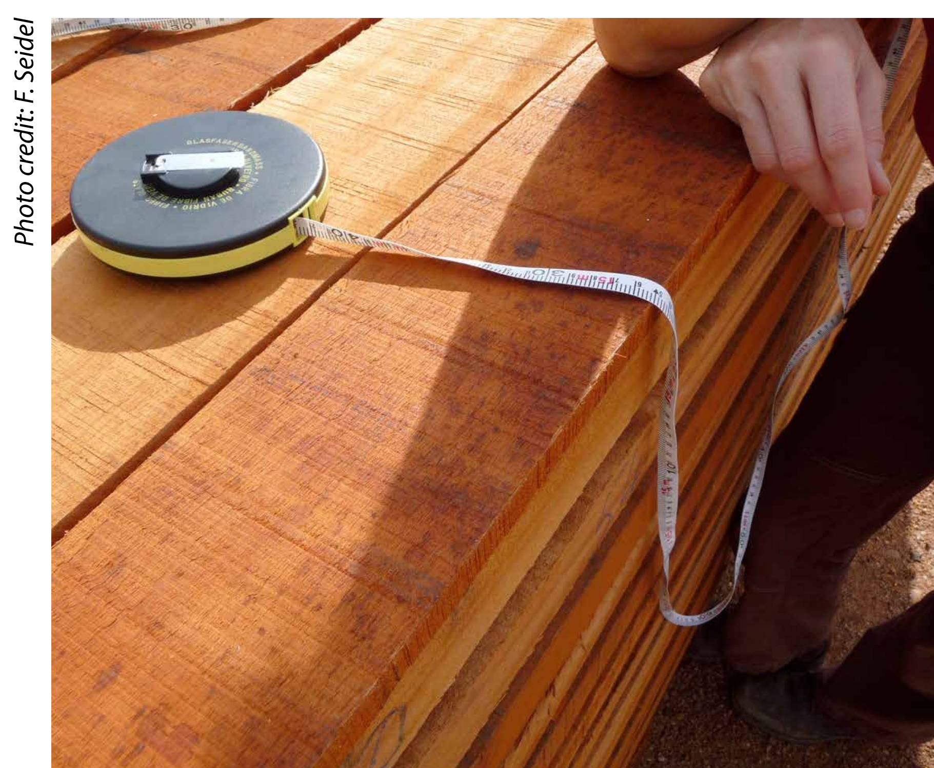
Measurement of a timber shipment
