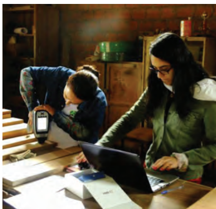
Wood identification using MicroNIRS and MicroPhazir devices. Photo: Alexandre Gontijo
