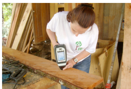
A portable NIRS device being tested in field conditions at a sawmill in Manoel Urbano, Acre state, Brazil. Photo: Jez Braga
