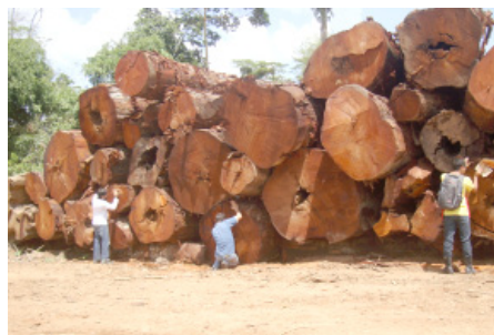
A field team preparing wood surface for obtaining mahogany's NIRS spectra at Fazenda Seringal Novo Macapá, Acre state, Brazil. Photo: Tereza Pastore
