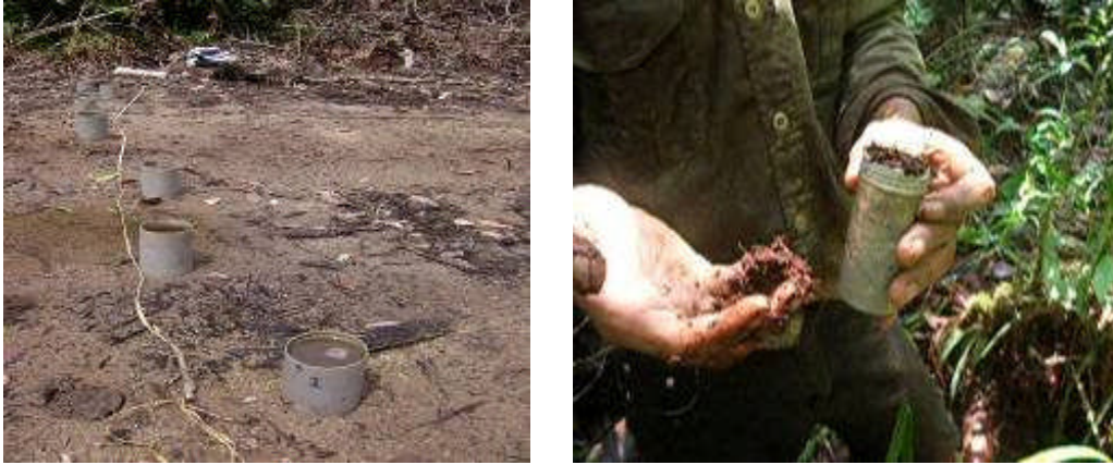
Figure 7.6 Measurements of infiltrations (left) and storage of peat soil in soil core tube for soil moisture sampling (right)
