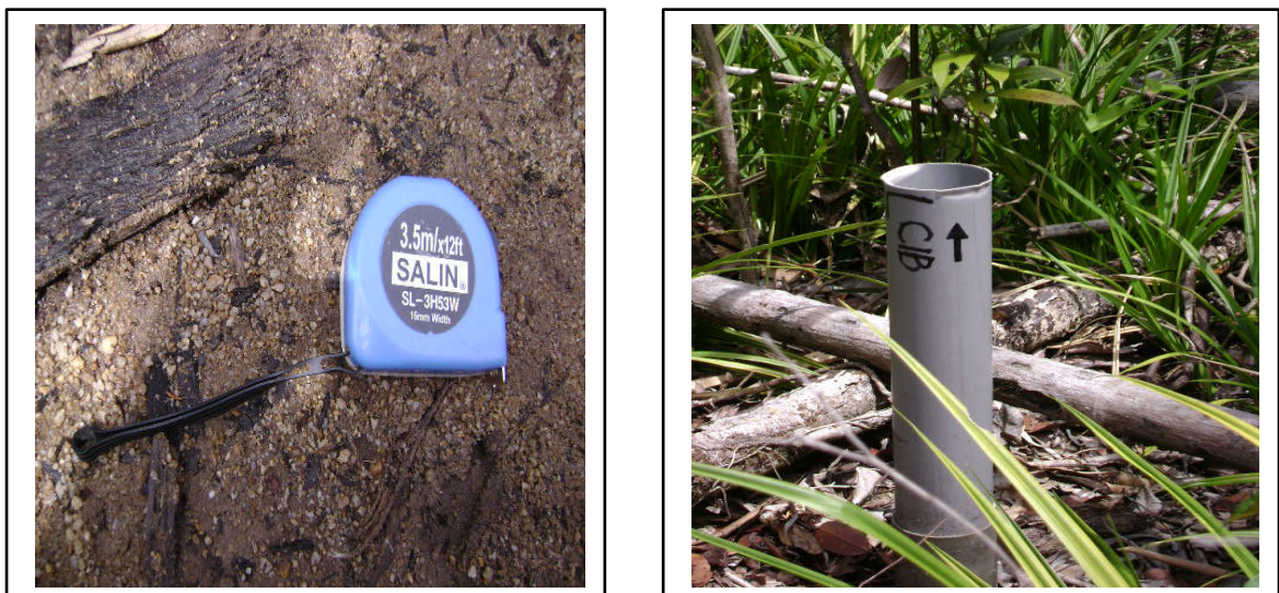
Figure 7.4 Measuring tape and PVC pipe to measure the groundwater level.
