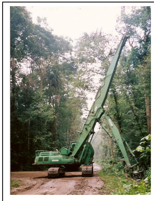
Figure 1.5 The Rimbaka timber harvester restricts its movement by pulling logs using a long cable hence minimizing the extraction damage to the forest floor
