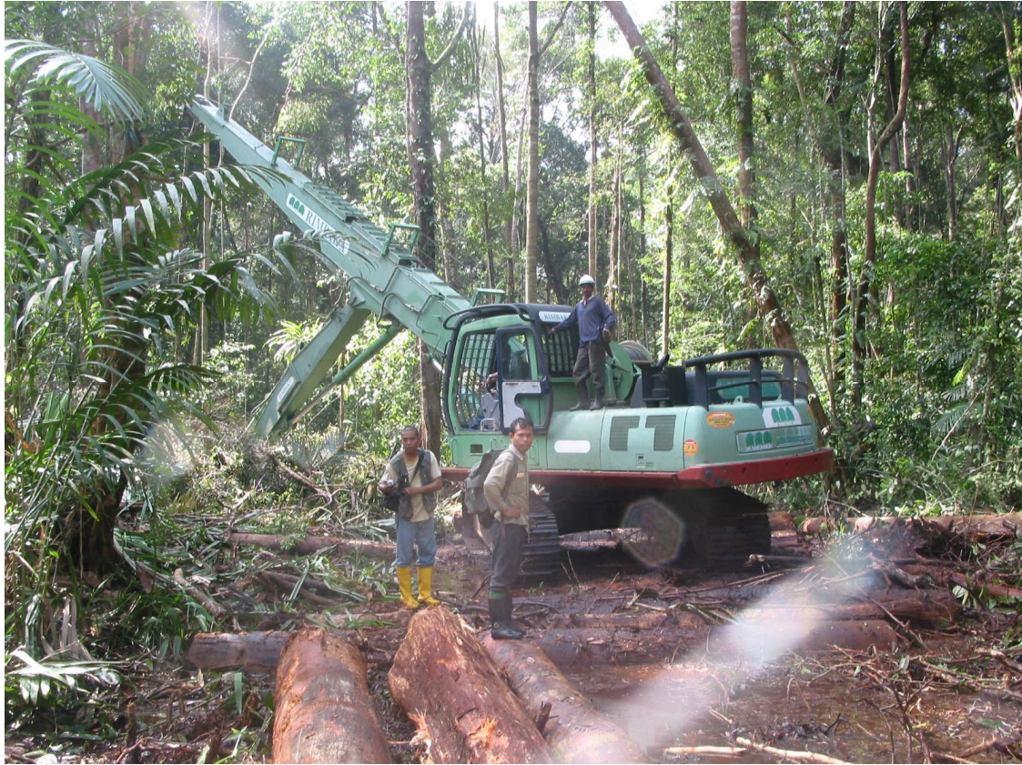
Figure 6 The Rimbaka timber harvester restricts its movement by pulling logs using a long cable hence minimizing the extraction damage to the forest floor
