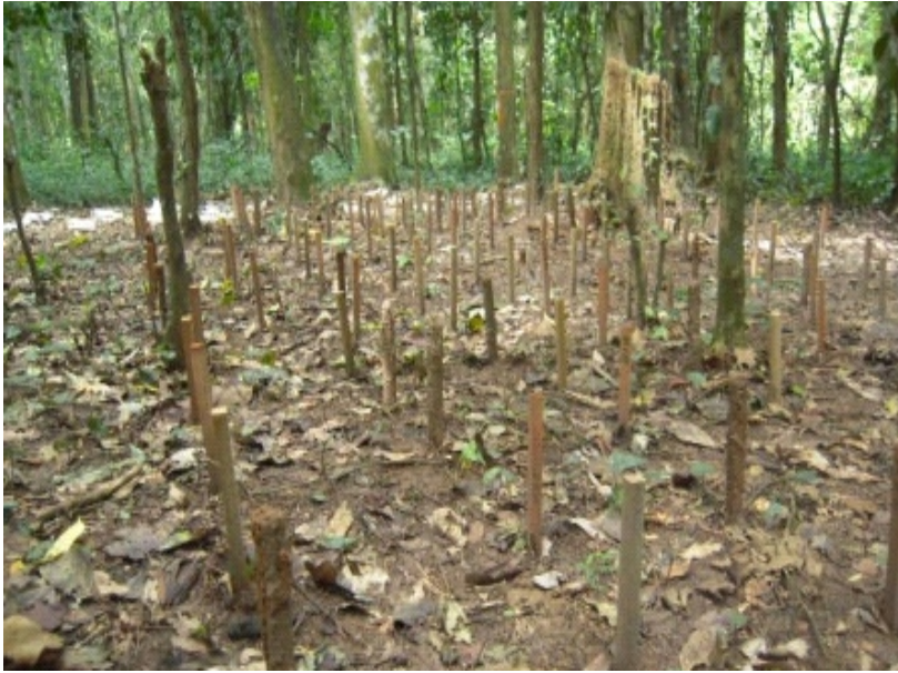
Fig. 9.8b: Stakes planted in graveyard test
