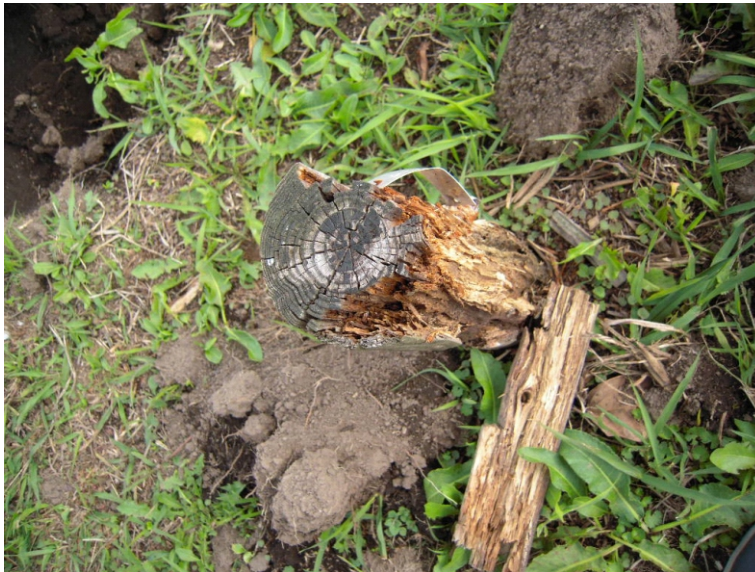
Fig. 9.7: Fungal attack and damage
