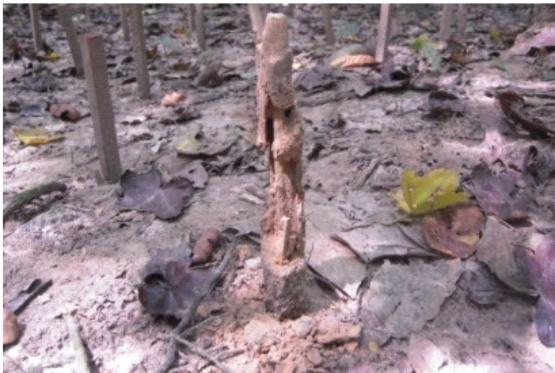
Figure 9.9: Termite attack in graveyard test
