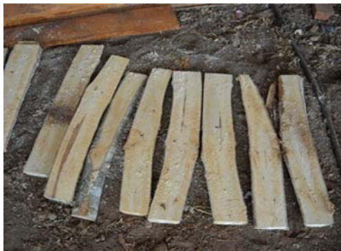
Result of multi-ripper sawing
