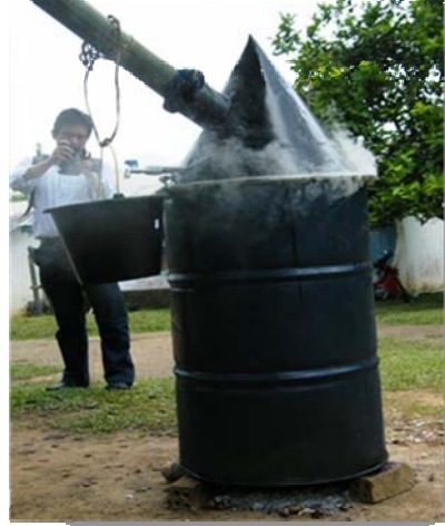
The complete structure of a charcoal drum kiln
