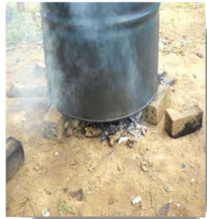
The complete structure of a charcoal drum kiln
