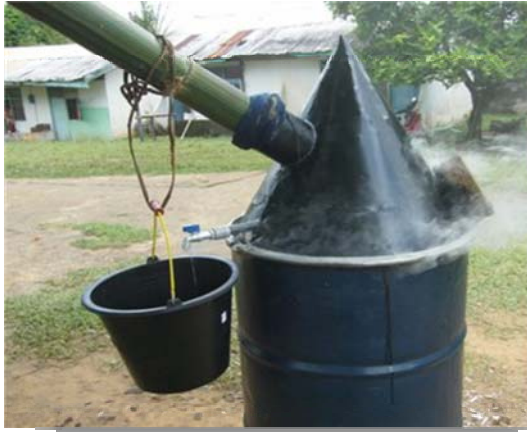
Wood-burnt residual smoke channeled to bamboo pipe
