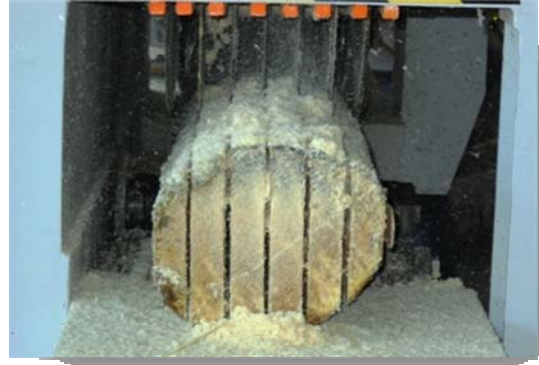
Multi-ripper sawing in progress
