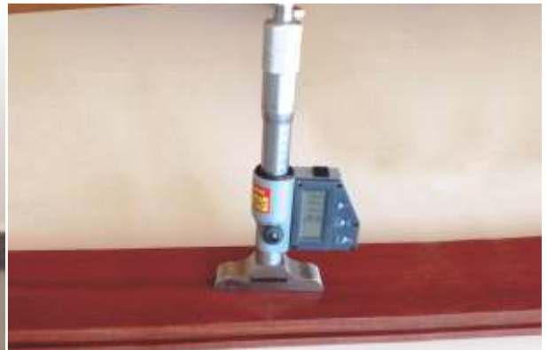
Impacto / Falling - ball indentation
