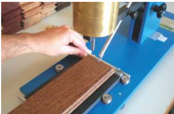
Risco / Scrape adhesion
