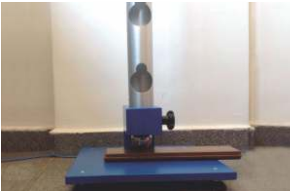
Impacto / Falling - ball indentation
