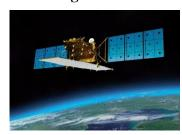
The state-of-the-art L-band Synthetic Aperture Radar-2 (PALSAR-2) aboard ALOS-2, which is active microwave radar using the 1.2GHz frequency range, have enhanced performance compared to the DAICHI/PALSAR in responding to society's needs. The PALSAR-2 can observe day and night around the clock.
