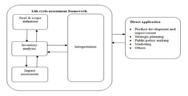
Fig. 1: The phases of an LCA according to ISO 14044 (2006)
