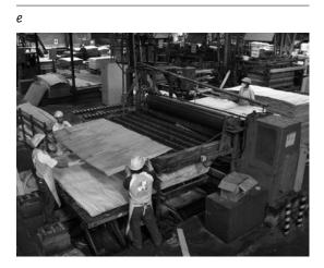
Two automatic trimming lines, one per mill, square each board to perfection (see Figure 80).
