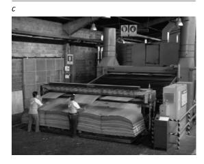
Six veneer dryers of different brands are in operation, three shifts per day, six days per week. Some are equipped with moisture meters at the dry end to avoid over-drying. A series of five core composers per mill are used to maximize recovery and quality.
