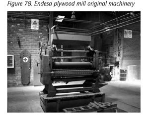
Since most of the machinery is imported, the weight of fixed assets is a lot more critical than in Japan, Europe or the US; therefore we must utilize old machinery as efficiently as possible. The Endesa team of engineers has been successful in modernizing these 30-year-old machines by changing electrical systems to electronic systems, improving material flows, and, where possible, automation.
