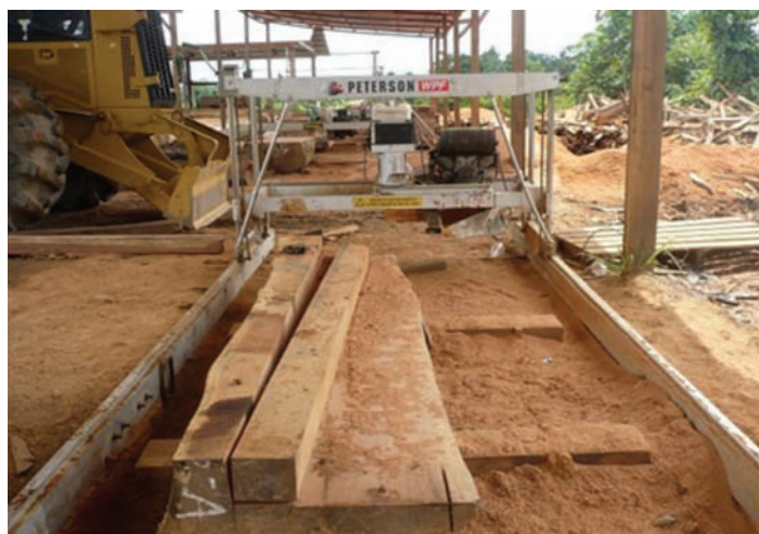
Bush saw: Portable sawmill at a sorting yard in Madre de Dios. Photo: Maderyja
