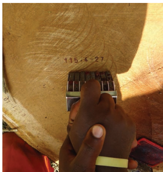
...and numbered: Device for numbering sawn timber. Photos: K.S. Bobo
