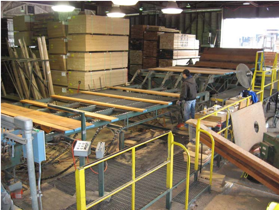
Px (g) Sorting line at distribution yard. Imported lumber is often custom graded for specific customers and/or end uses.
