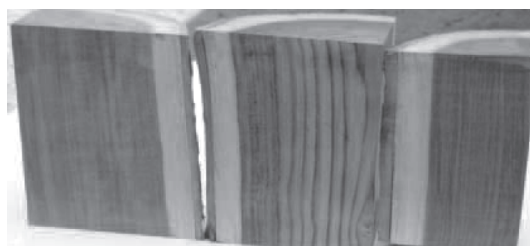
Fig. 1. Heartwood colour difference between homestead and plantation teakwood. Note the paler heartwood in sample from wet site (left), golden brown colour with black streaks in dry site (middle), and uniform golden brown colour of forest plantation teak (right).
