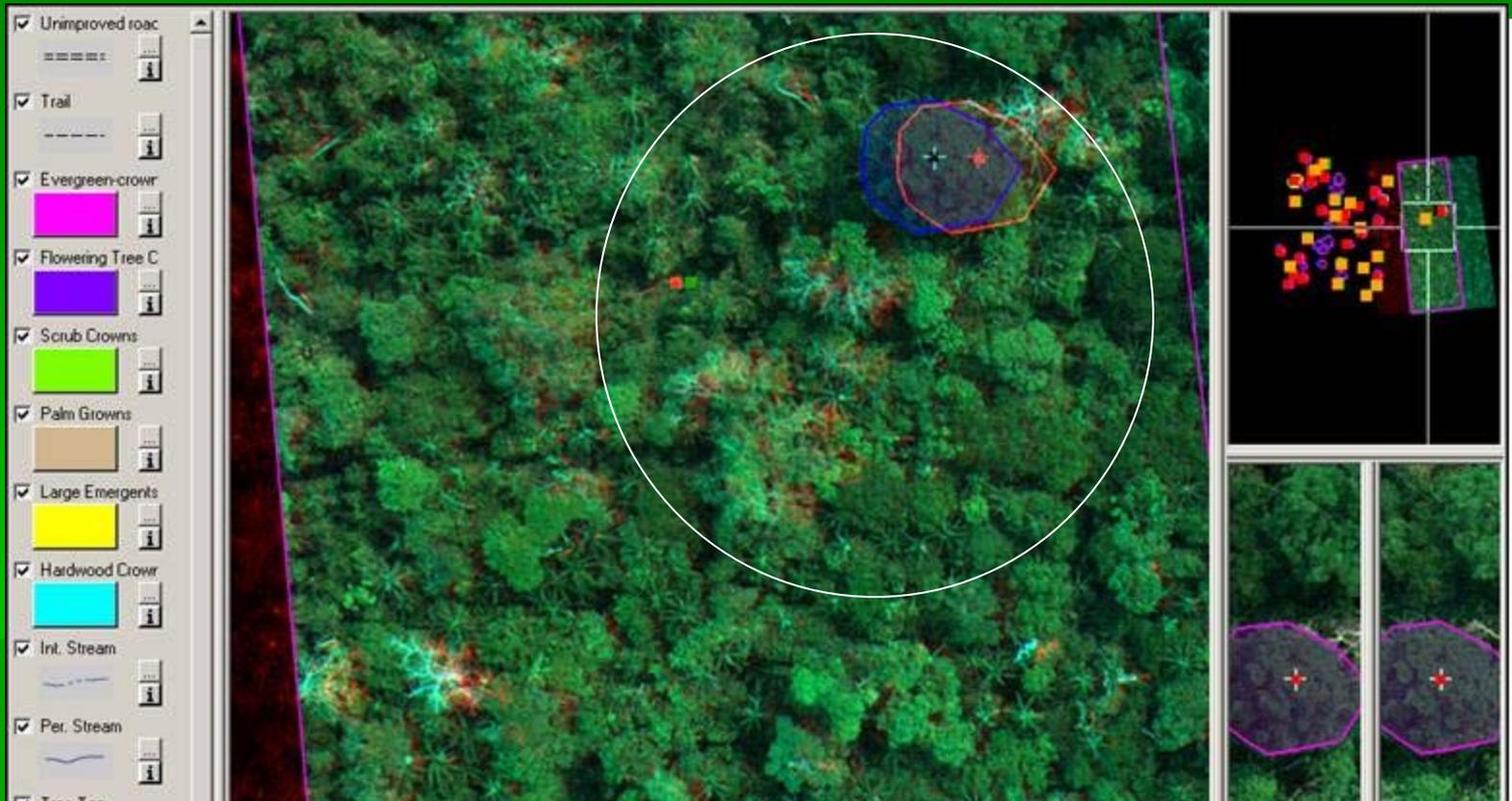
Individual trees are measured for height, crown area, and in some cases species—combine with equation of biomass of tree vs crown area x height or crown area alone
