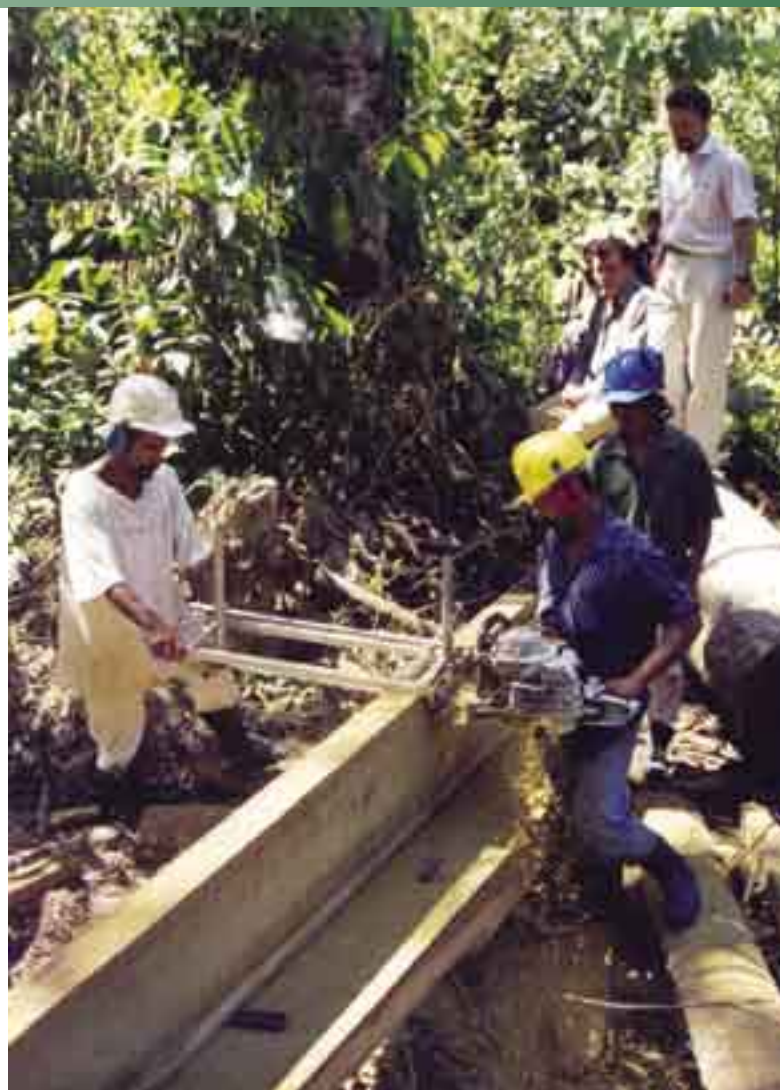
Framework: project officers assess the practicability and efficiency of chainsawing with frames.
