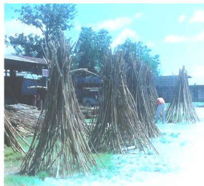
Fig. 4. “Wigwam” form of drying rattan poles
