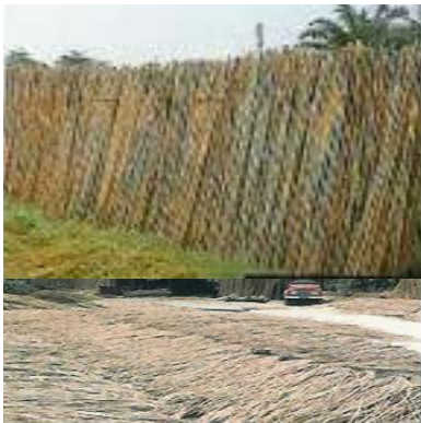
Fig. 3 Air drying of rattan poles in near vertical (top) and horizontal position (lower photo)
