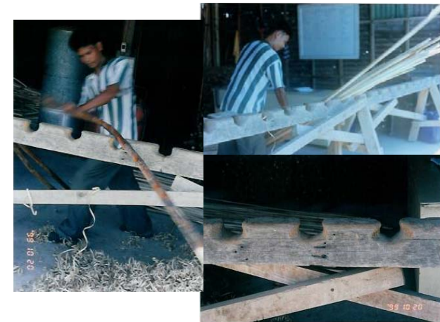
Fig. 13. A straightening gadget made of wood.
