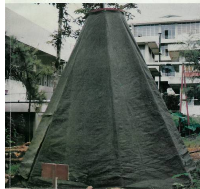
Fig. 6. A portable and demountable kiln dryer designed for drying rattan poles near or within the cutting site (Casin 1985)
