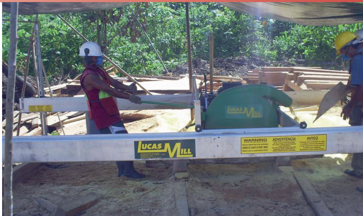
Beats pit-sawing: Portable sawmill in Asháninka community, Peru (PD 14/96 Rev.1 (F)). Photo: A. Gaviria
