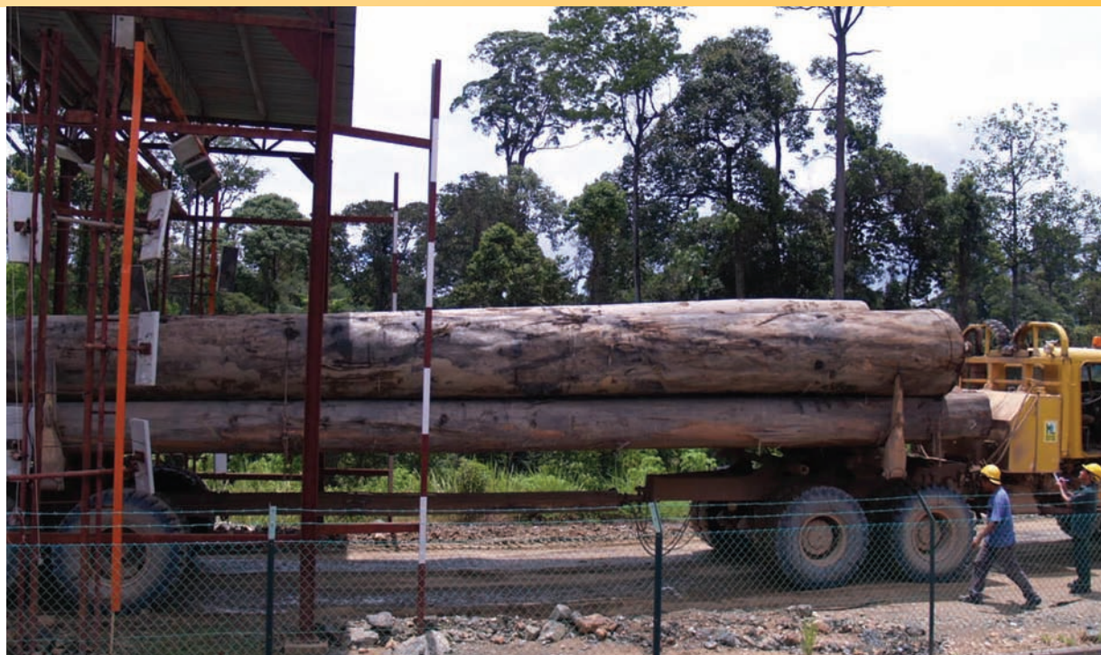
Radio tagged: RFID gantry in Sabah monitoring log movements. Photo: B.H. Ghazali
