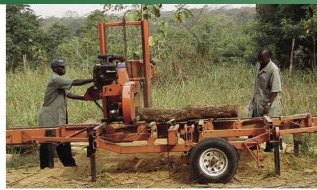
**Economizing:** the horizontal mobile bandmill known as the woodmizer was used for the primary breakdown of branchwood into lumber. *Photo:* © *R. Okai*
