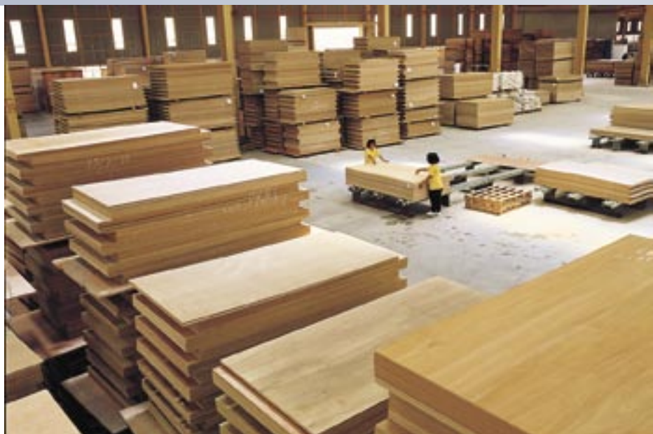
Stacked: plywood sheets in Sarawak, Malaysia, stacked for curing and inspection prior to export. Photo: courtesy Samling Corp
